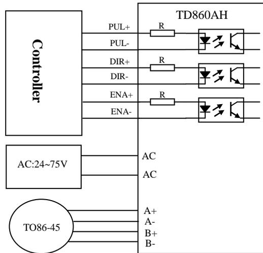
Figure 9 TD860AH Typical connection
