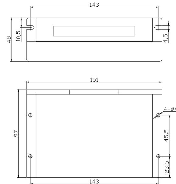
Figure 1: Mechanical specifications
